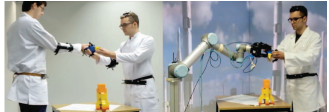
Fig. 1. From motion captured human-human demonstrations an interaction model of a cooperative task is learned. Using the learned model in a human-robot collaboration, the robot's behavior is continuously synchronized, both spatially and temporally, with the actions of the human.
