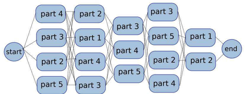
At run time, the interaction network is transitioned independently by the robot. It chooses one of the actions in each layer while maintaining its ability to finish the task by not selecting actions twice or blocking itself from further execution.
