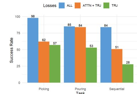
**Losses:** We utilize auxiliary losses to complement the generated robot control signal. Guiding the **object detection (ATTN)** helps in the pouring task, guiding the **policy generation** yields significant performance increases in the pouring task.
